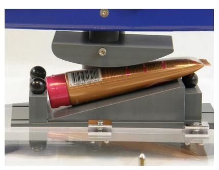
The tube seal tester ATS is the tool for checking the seal strength of plastic and metal-plastic tubes.
